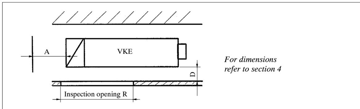
R: Inspection opening to grant access to the unit (especially the electric and the water connections) for maintenance and installation must be provided
