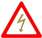
Electrical operation of the unit in a partly disassembled condition or of individual components is not permitted since earth terminals might be interrupted.
