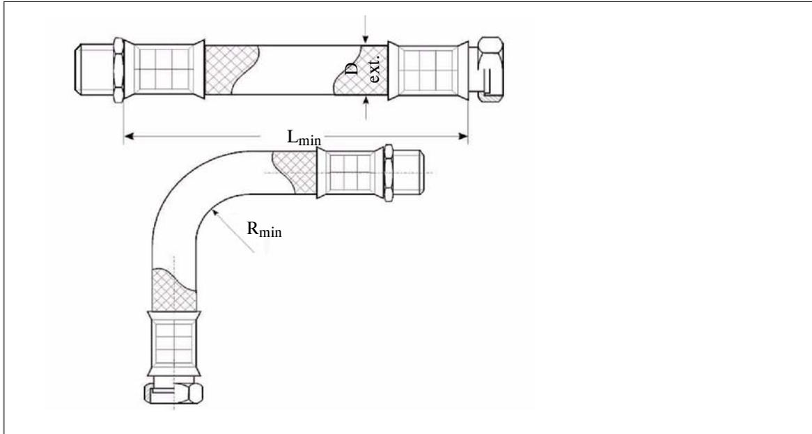
**Armoured hose Oxystop up to +70 °C (diffusion inhibiting, marked through weaved-in blue strip)**
