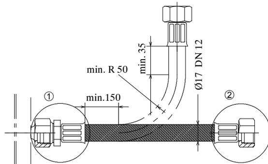
Hose without insulation. For insulated hoses, dimensions will change accordingly.
