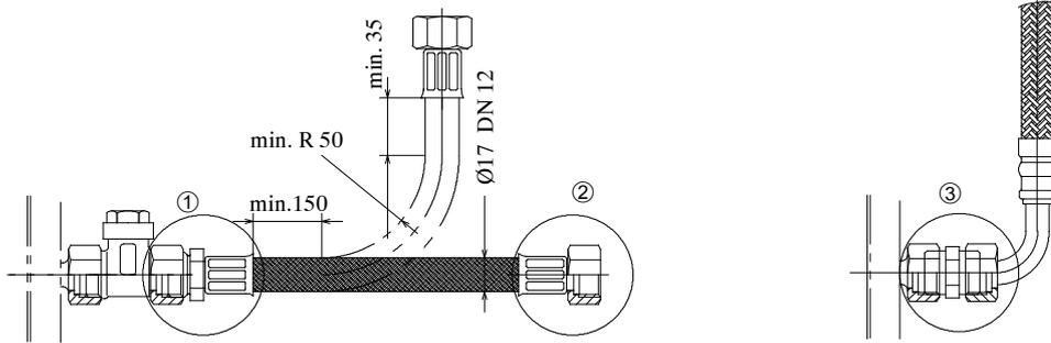
Hose without insulation. For insulated hoses, dimensions will change accordingly (10 mm Armaflex insulation).
