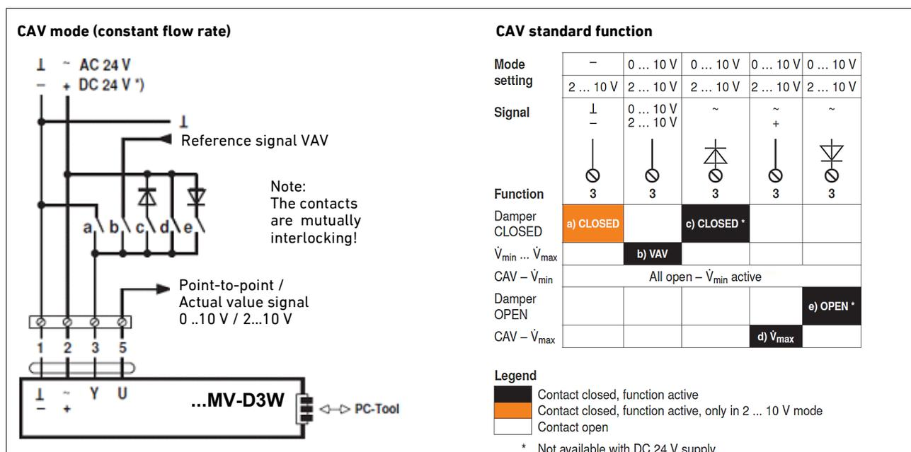
Wire diagrams for other control components on request.
