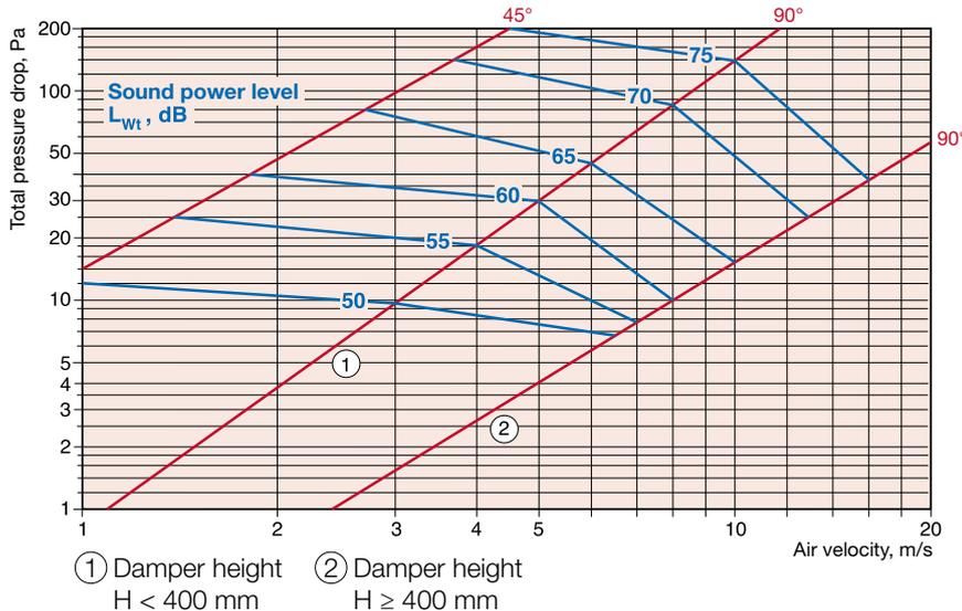
The speed is calculated on the damper's gross area, i.e. a BSK6R - 400 x 400 has a gross area of 0.16 m<sup>2</sup>.
