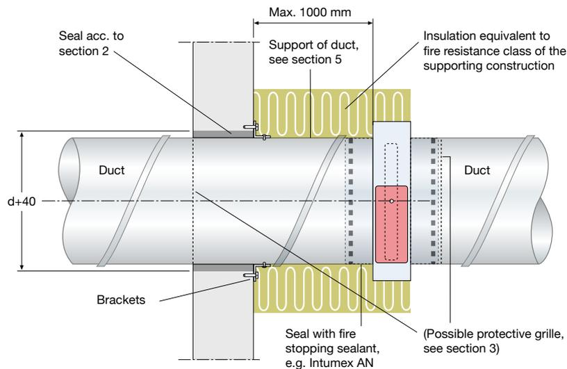
1. Install the damper in the duct.
