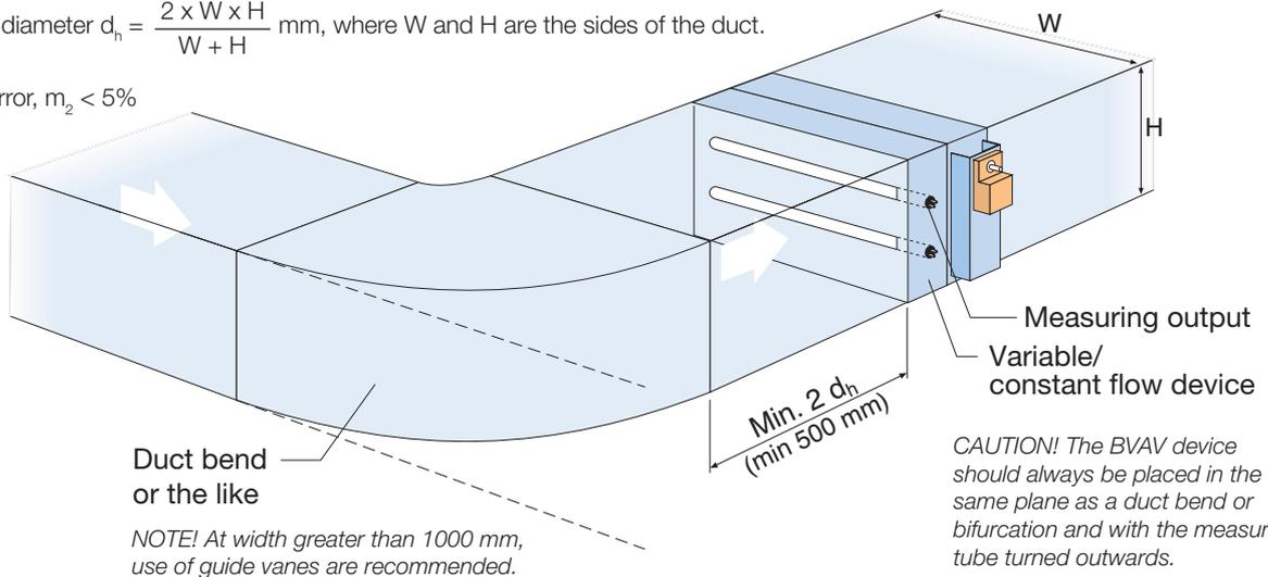
**NOTE!** At width greater than 1000 mm, use of guide vanes are recommended.
