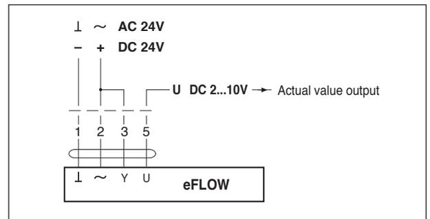
**Control functions for eFLOW-actuator**
