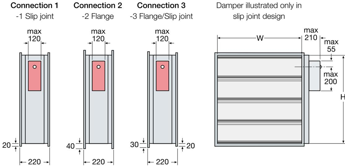
RABR for installation in combination with RBVG supplied with connection type 3 Slip joint/Flange. RABR 250, 450, 650 etc. in height is supplied with a raised slip joint or flange connection.
