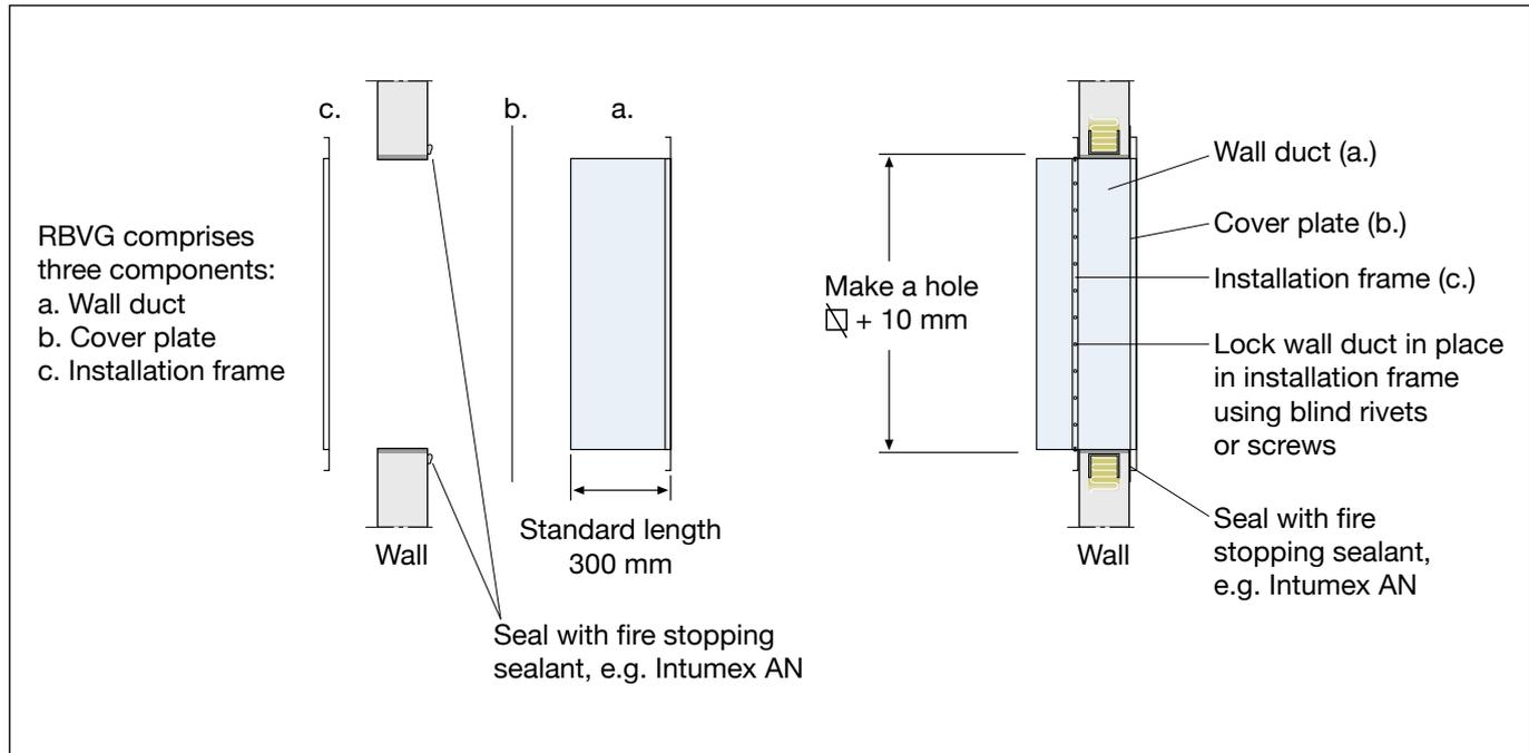
1. Make a hole, corresponding to the duct's nominal dimensions + 10 mm, in the building element.
