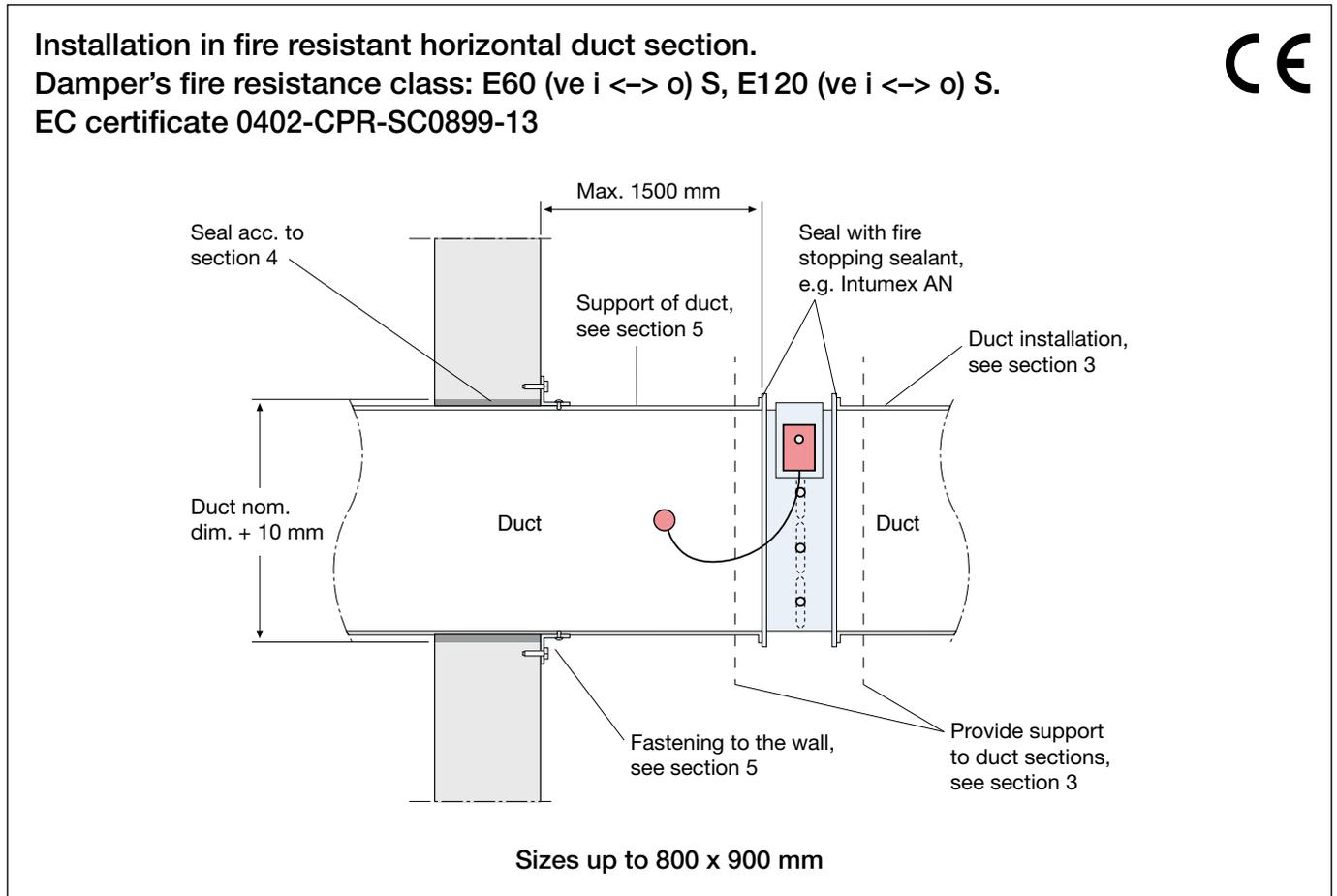
1. Install the damper in the duct with connection for slide joint or flange. Seal with fire stopping sealant, e.g. Intumex AN.
