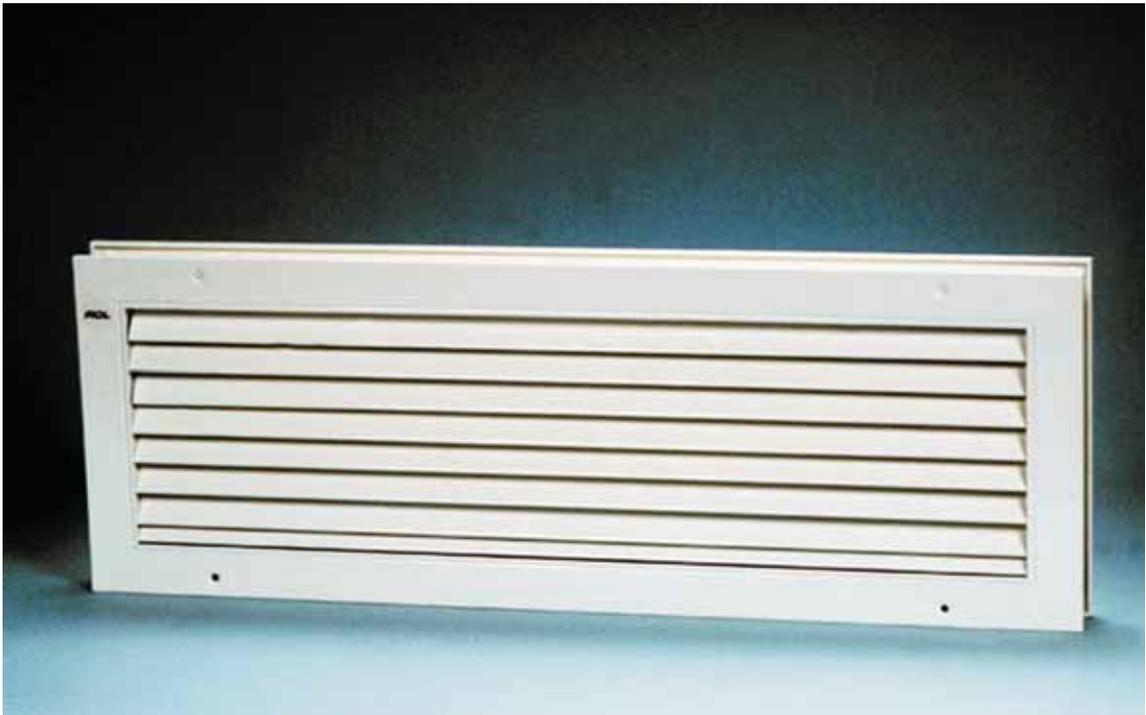
Transfer air grille between two rooms. Can be installed either in the door or in the wall, recommended installation depth is 30-50 mm. When thickness of the construction is more than 50 mm has one door grille to be installed on both sides. No visibility through the grille. Free area is approximately 50 %.
