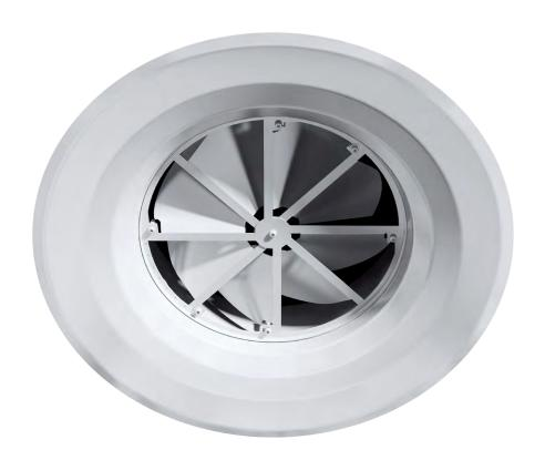
RIF is suitable for ventilation, heating and cooling in high spaces. The throw pattern is adjustable from horizontal to vertical by changing the vanes position, either manually (RIF) or with an actuator (RIF-M).
