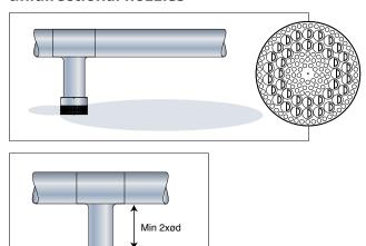
Thanks to its flexibility, **RUX** is a perfect choice for spaces in which the layout may change during their lifcycle. If, for example, a work station, shelf or freezer box is installed underneath the vertical throw pattern, the throw may be easily redirected towards free floor space simply by turning the nozzles.
