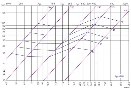
Sound absorption area: Size 160-200: 10 m<sup>2</sup> Size 250-315: 15 m<sup>2</sup> Size 400: 20 m<sup>2</sup>
